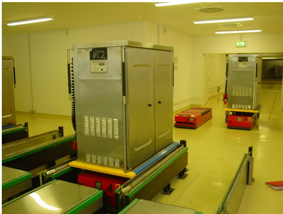
handover module to the AGVs
